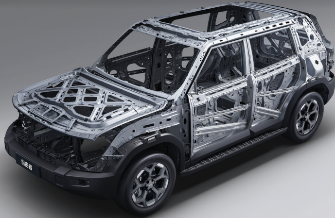
Reinforced Body Structure
